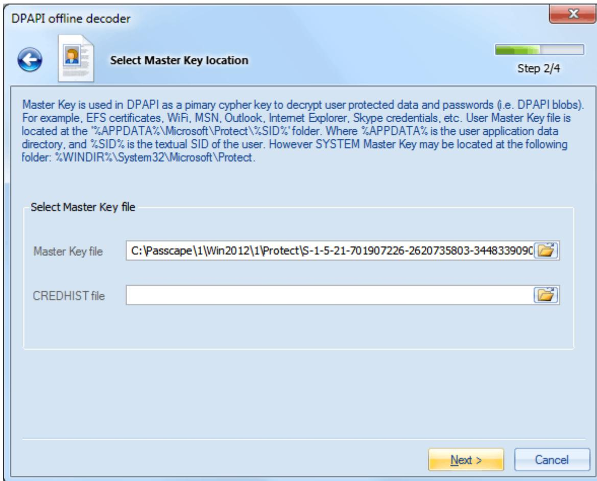
On the second step of the Wizard, specify the path to the data owner's Master Key: select the path and then click Next. The program pops a warning that a vulnerability is found in the Master Key, and therefore the decryption can be carried out two ways: with the user's password and without it. We, certainly, want the latter.
